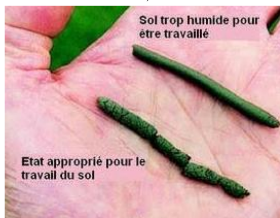
Figure 7 : Test du crayon (Shepherd, 2000)
